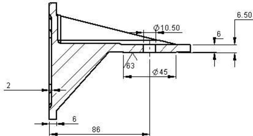
**Figure 2: Tilt mount base – Side View**
